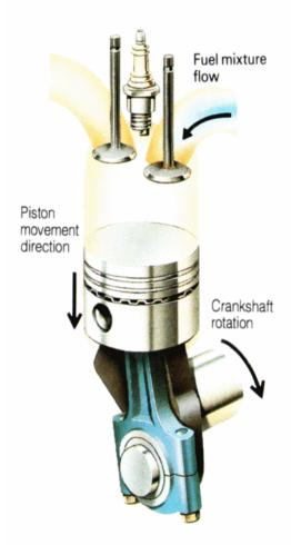
On the induction stroke the piston is descending, the inlet valve is fully open and the exhaust valve closed.
