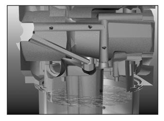
The second path is when dirt or debris enters from the fuel system and travels through the pilot jet orifice to the transition ports.
