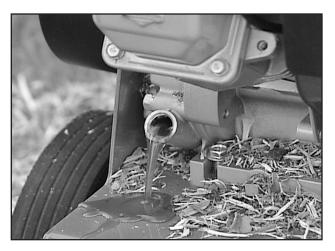
down the cylinder wall, and into the crankcase. This condition is called "cylinder wall wash" and will eventually cause a failure of the piston rings and cylinder wall.
