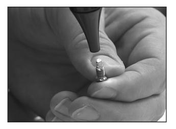
Dirt and debris entering through a ripped or torn air cleaner can collect in the idle air circuit causing it to become clogged before the pilot jet. When this occurs the pilot jet will only flow raw fuel to the combustion chamber from idle to light load conditions. This can result in light black smoke from the exhaust. The carburetor will hunt and surge due to this symptom. An otoscope is a great tool to help diagnose this condition.
