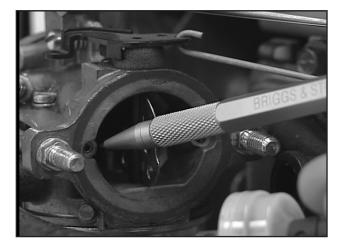
To isolate whether the problem is carburetor or governor related, hold the throttle plate closed to force the engine to idle. If the engine continues to run, you know there's a problem with the governor system. If the engine stalls, inspect the fuel supply route to the idle circuit. The smallest fuel orifice in most float feed style carburetors is the idle circuit pilot jet.
